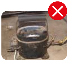
FIGURE 8: COMPRESSORS MUST NOT BE USED FOR VACUUMING
