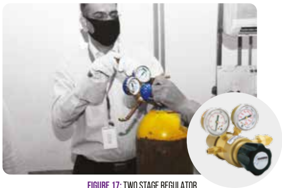
FIGURE 17: TWO STAGE REGULATOR
